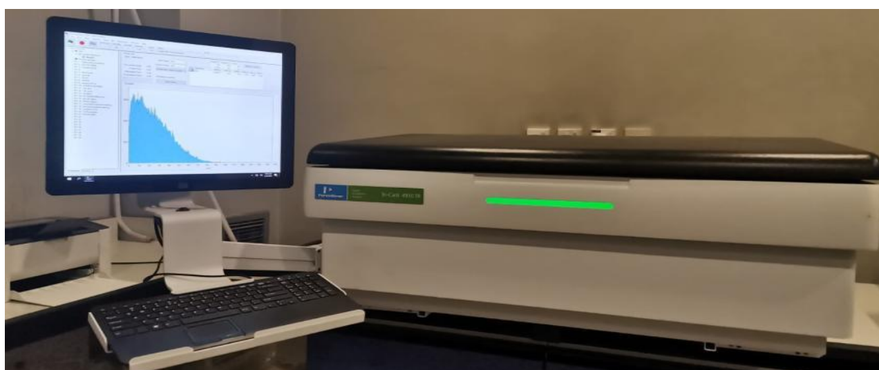
Fig (2) B Canberra Packard 4910 TR liquid scintillation analyzer and spectrum of gross Alpha and Beta
